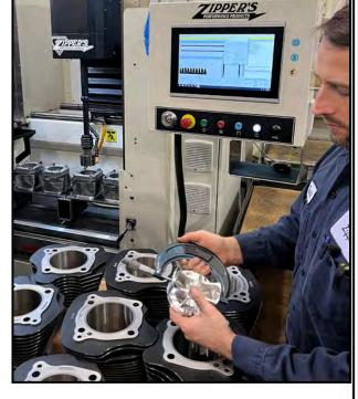
Zipper's M8 Big Bore Kits are a Cut Above the Rest! Some outfits sell M8 big bore kits where they source a finished-sized cylinder from one vendor and a piston from another. This will never happen at Zipper's. Our big bore cylinders are manufactured to our specs, with oversize cast iron liners and undersized bores. Our experience in sizing cylinders for a straight and true bore dictates that they are:
